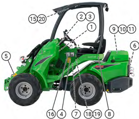
Labels on loaders with ROPS canopy
