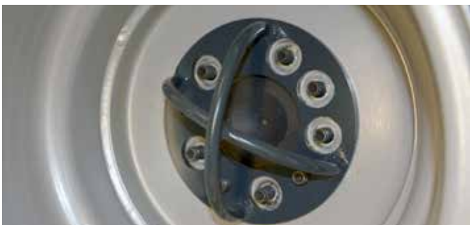
Tie down bracket on wheel hub A423091
