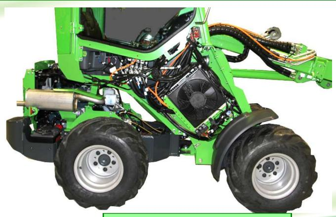
The orange line illustrates the routing of the cable harness, how it should be installed
