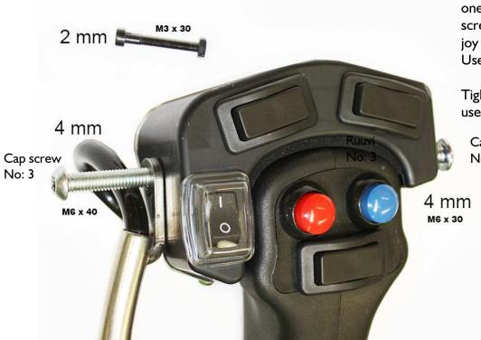
Before fitting the screws No: 2. ja 3. one must remove the original fastening screw M3 x 30 from the top of the joy stick handle.
