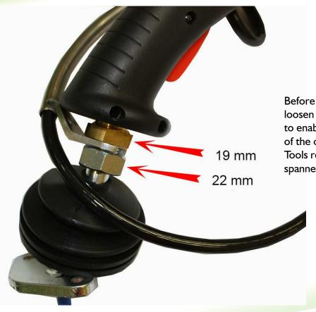
Before attaching the control panel, loosen the fastening nuts of the joy-stick to enable pushing in the cable support of the control panel.
