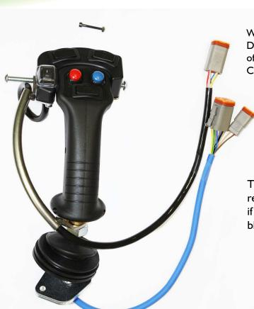
When the installation is ready one must connect the DIN socket of the black cable, to the cable harness of the Attachment Control Switch Pack.
