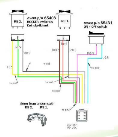
These are the switches for the additional control panel p/n A34716
