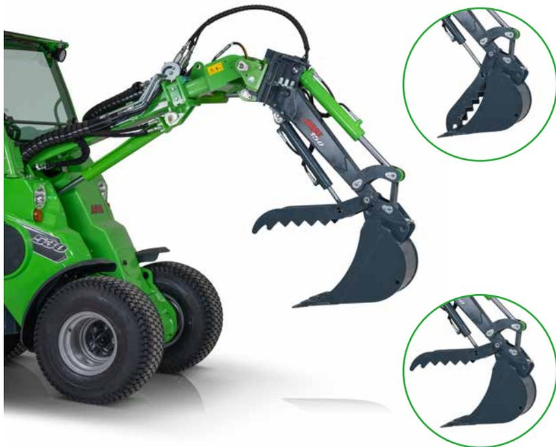
Hydraulic thumb grab is now available as an option also for the mini digger 150. The thumb grab can be mounted on mini diggers 150 made in January 2021 or later, and the thumb grab can also be retrofitted to older mini diggers by drilling holes for thumb grab cylinder brackets to the digger arm.
