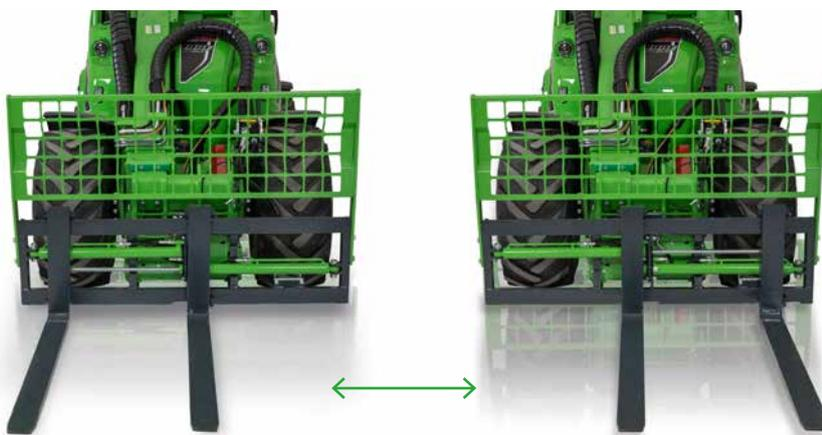
The 2000 kg capacity HD pallet fork with hydraulic side shift and fork width adjustment will be available in May. It is equipped with 1200 mm long forks, and the load support frame is standard like on the 1200 kg model.
