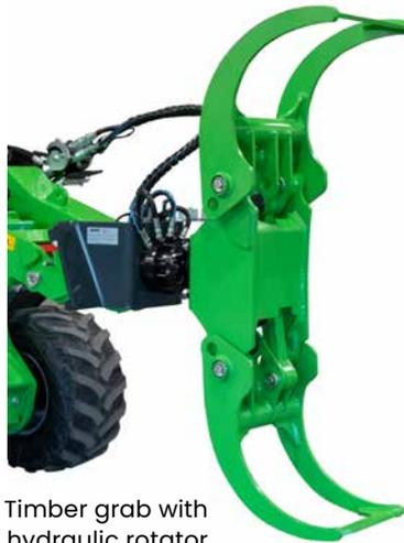
Timber grab with hydraulic rotator
