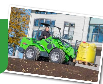
ith its 1900 kg lift capacity and 3.5 m lift height (half a metre longer than the Avant 700 series), the new Avant 800 series definitely stands out among compact loaders. As with other Avant loaders, the 800 series comes equipped with hydrostatic transmission with a hydraulic drive motor on each wheel with two drive speed areas. The drive speed of the 800 series maxes out at 30 km/h.
