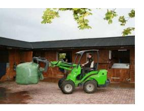
and a useful lift capacity of 1000 kg. In addition, like all Avant machines, the 630 has an offset, self-levelling telescopic boom which not only ensures excellent handling capabilities but also provides the driver with an unrestricted view of the attachment for maximum safety in use.
