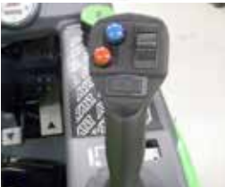
A37093 Hand drive controls • With this system you can operate the forward-reverse drive from a switch on the joystick or use the standard pedals. Selection between hand drive and drive pedals is as easy as a flip of a switch on the dashboard.
