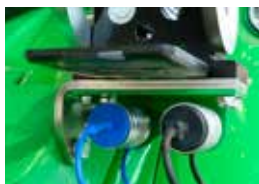
A35504 Extra aux. hydr. double acting outlet front, 400 series For customers who want to mount the tilt adapter (must be equipped with conventional type quick cou- plers) and a hydraulic attachment – like 4 in 1 bucket - on the machine at the same time.
