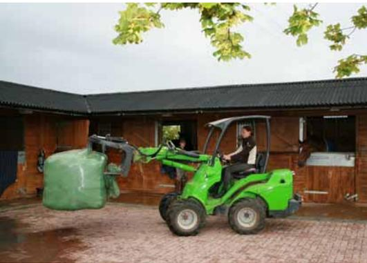
and a useful lift capacity of 1000 kg. In addition, like all Avant machines, the 630 has an offset, self-levelling telescopic boom which not only ensures excellent handling capabilities but also provides the driver with an unrestricted view of the attachment for maximum safety in use.
