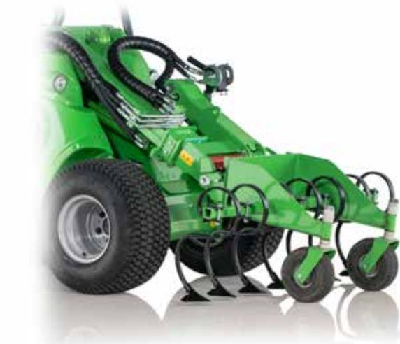
The front cultivator can be used for instance together with the horse arena harrow. Especially useful in a more compacted arena or an outdoor riding area. It is equipped with large tines which loosen the soil and make harrowing of the arena easier. Equipped with two wheels in the front.
