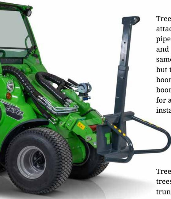
Tree boom is a simple and practical attachment for handling bigger tree trunks, pipes etc. objects which need to be lifted and placed with accuracy. It is otherwise the same attachment as the Avant big bag lifter, but the manually adjustable telescoping boom doesn't have a hook – instead the boom is straight and equipped with a pin for attaching lifting slings. This allows, for instance, lifting and planting bigger trees without the risk of damaging them.
