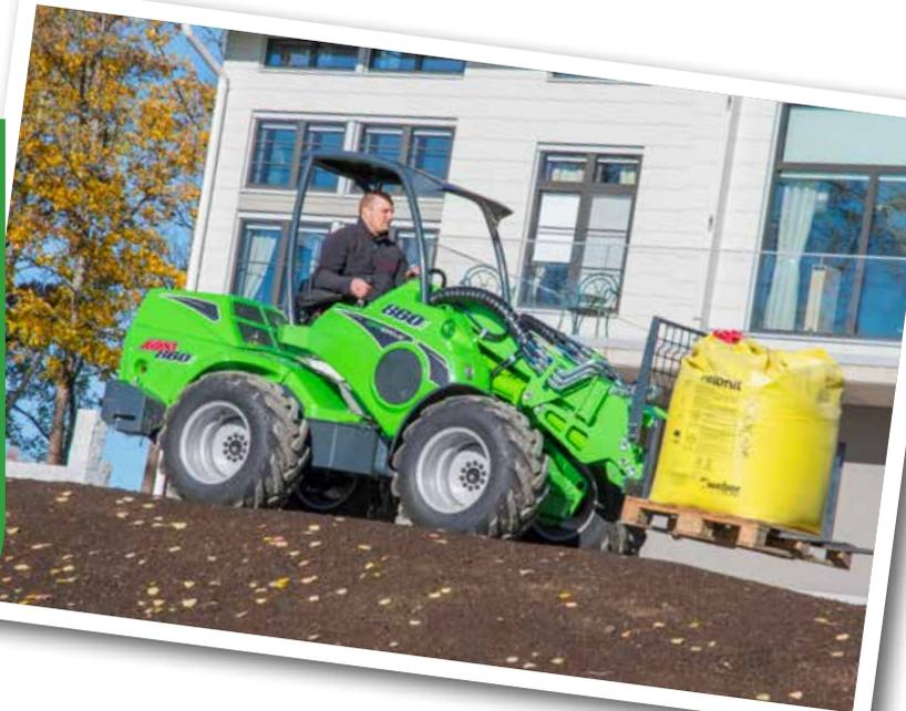
With its 1900 kg lift capacity and 3.5 m lift height (half a metre longer than the Avant 700 series), the new Avant 800 series definitely stands out among compact loaders. As with other Avant loaders, the 800 series comes equipped with hydrostatic transmission with a hydraulic drive motor on each wheel with two drive speed areas. The drive speed of the 800 series maxes out at 30 km/h.
